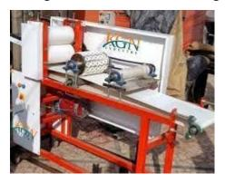
• Cutting Machine: Cuts the dough sheets into round or square papads.
