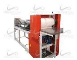
• **Drying Chamber:** Used to dry the papads evenly and quickly, especially during humid weather.
